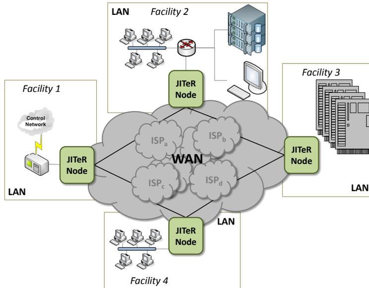
Figure 1: WAN-of-LANs model of an information infrastructure using JITEr.
